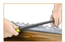
Once this is done, the same process should be applied to the remaining gaps, but with the point of the file tilted 15° towards the handle.
