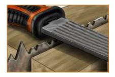
The process for sharpening crosscut saws is very similar to the one used to sharpen rip saws.
