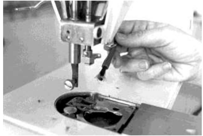
Figure 4. Bobbin area. Clean carefully to remove lint using a soft brush. Tweezers may be helpful in removing stray threads.
