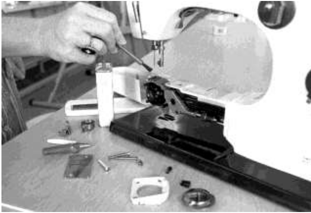
Figure 1. Remove all the parts possible in order to clean the machine thoroughly. Keep the parts in order to make it easier to replace them.
