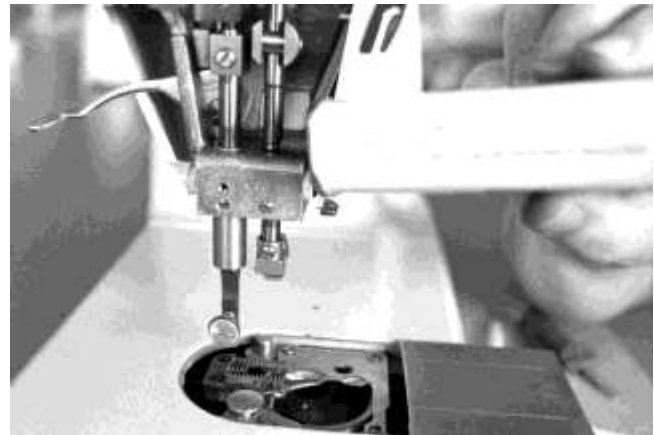
Figure 6. Face plate area. Place a drop or two of oil on moving parts where they slide through a housing or move against each other.
