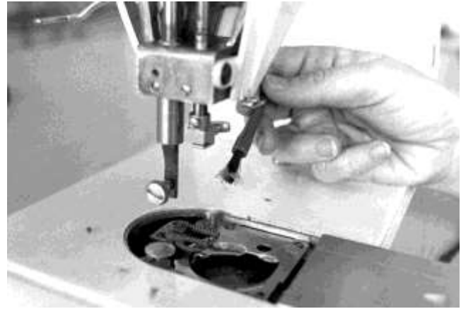
Figure 2. Bobbin area. If possible, remove the bobbin case to remove all lint and stray threads.
